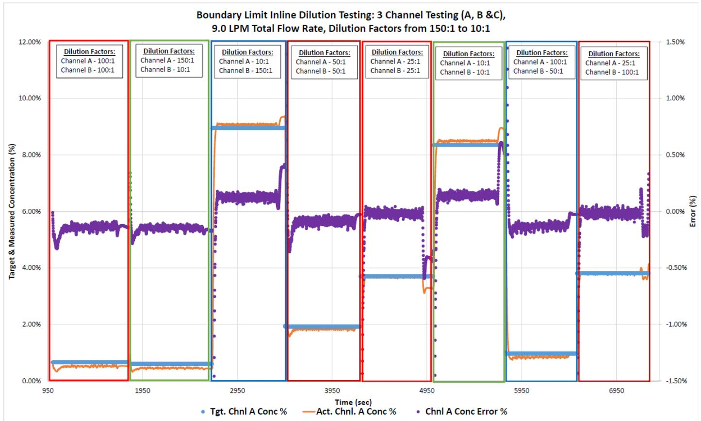
Figure 4. EcoPrime LPLC Enhanced BID Dilution Factors (10x, 25x, 50x, 100x, and 150) and associated Error % (concentration).
