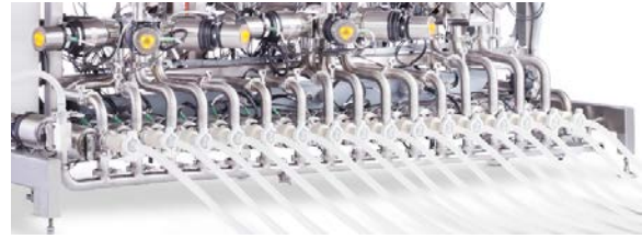
Figure 4: A proprietary buffer, feed and CIP manifold maintains an aseptic, closed environment between single use equipment and the Contichrom TWIN.
