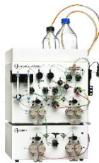
Contichrom HPLC equipment for peptide and oligo purification (ChromaCon)
